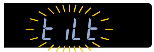
Warning that the balance is not level
