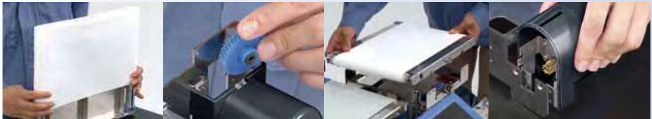
Replacing a belt
