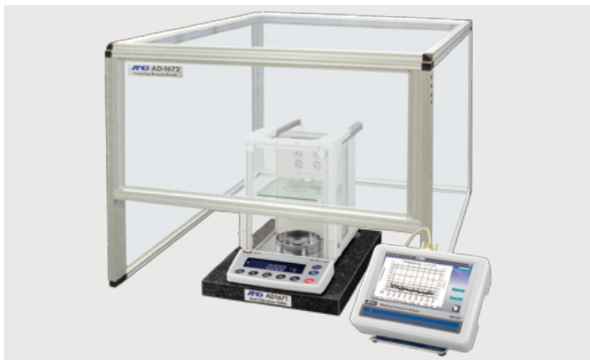
Taking data from the BM-20 microbalance
